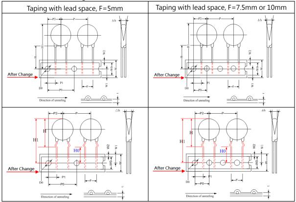
Models included: All models of varistor with taping.
